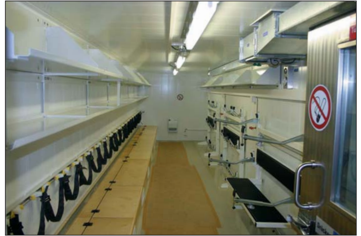
The rescue compartment. On the left are storage racks for helmets, breathing apparatus and other equipment. In rescue operations the boxes can be used as benches. On the right are special supports for stretchers together with folding benches.
